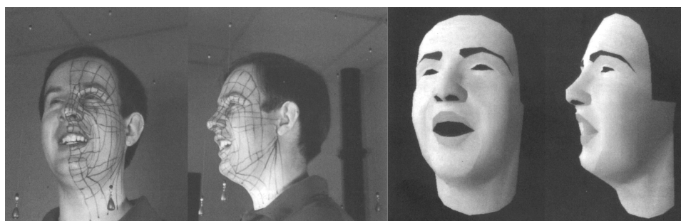
Figure 2.10: Reconstruction of a face in 3D by photogrammetry. The lines painted on the face facilitate establishing correspondences between multiple images, and also define the polygon topology of the 3D model (images from Parke, 1974).
