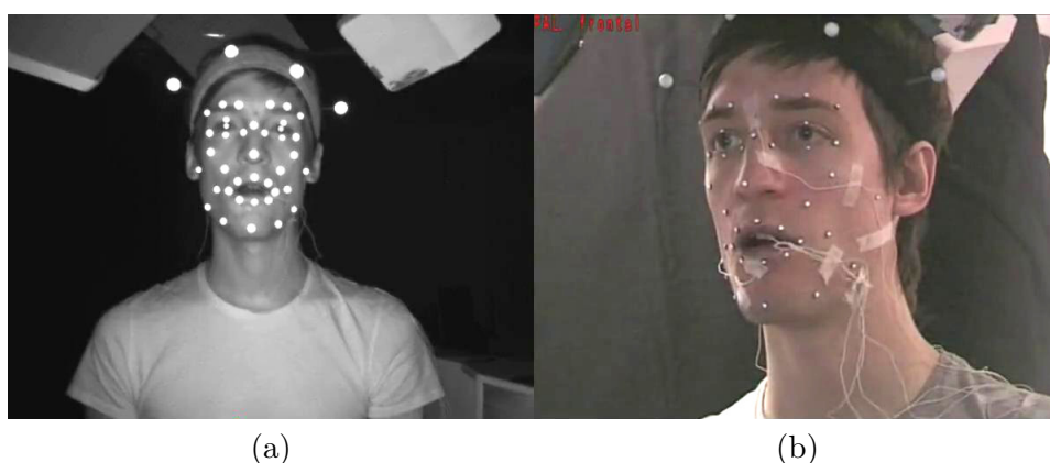
Figure 5.3: Example frames from the gray scale video from the OptiTrack system (a) and the color video from the camcorder (b).
