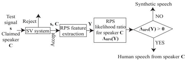
Fig. 8. Proposed system for detection of synthesized speech after speaker verification using phase-based detection.
