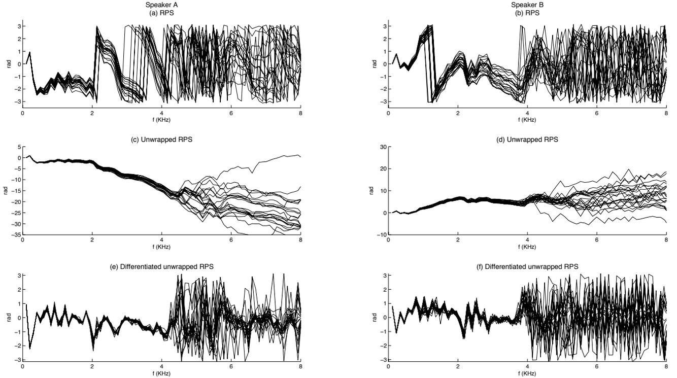
Fig. 6. RPS information for two sustained —i— speech segments of 200ms (20 frames) by two male speakers: (a-b) RPS, (c-d) unwrapped RPS, (e-f) differentiation of the unwrapped RPS
