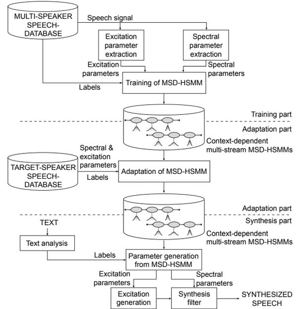
Fig. 2. Overview of the HTS-2008 speech synthesis system, which consists of four main components: speech analysis, average voice training, speaker adaptation, and speech generation.
