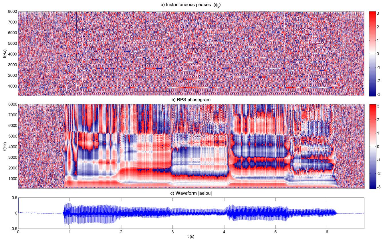
Fig. 5. Phasegrams of a voiced speech segment for five continuous vowels. a) Instantaneous phases b) Relative phase shift c) Signal waveform
