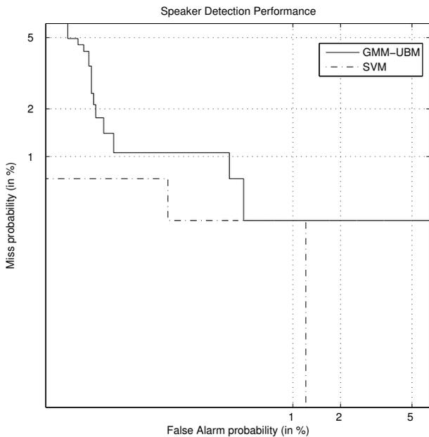
Fig. 9. DET curves for speaker verification using test signals from human speakers. The EER is 0.35% for GMM-UBM and SVM systems.
